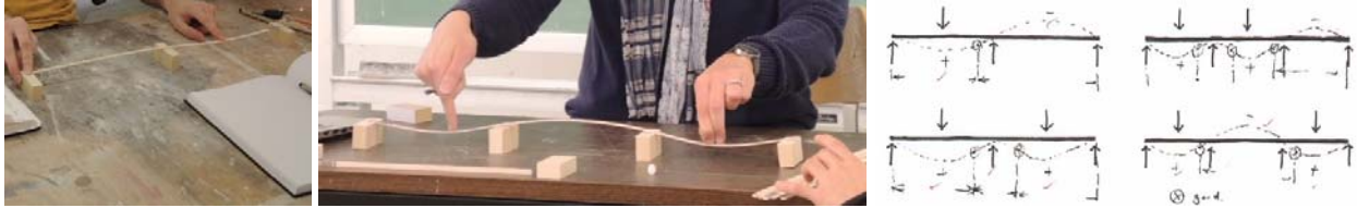
Fig. 6: A continuous beam over three supports (left), over four supports (middle), recording of the deflected shape by the students(right)
