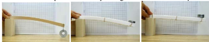
Fig. 5: Performance advantage of flitched beams
